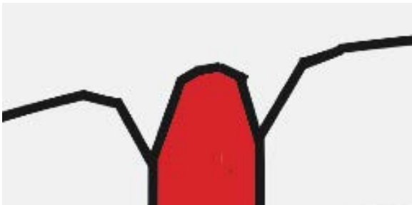
3 - Facet the top corners of the Vee Grooves
