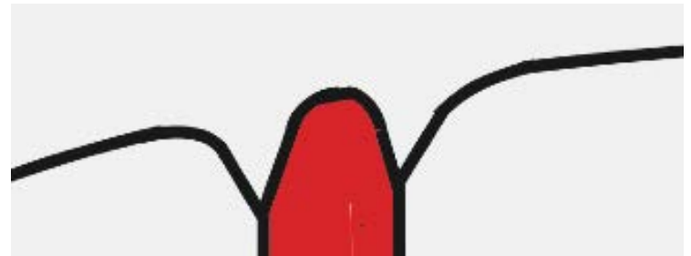
4 - Sand into a round bead shape
